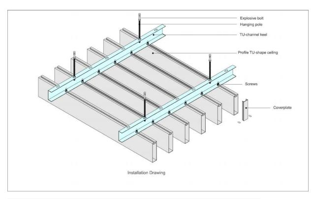
Profile TU-shape ceiling is a kind of visible type ceiling, and the visible angle of the installation area can be adjusted,
